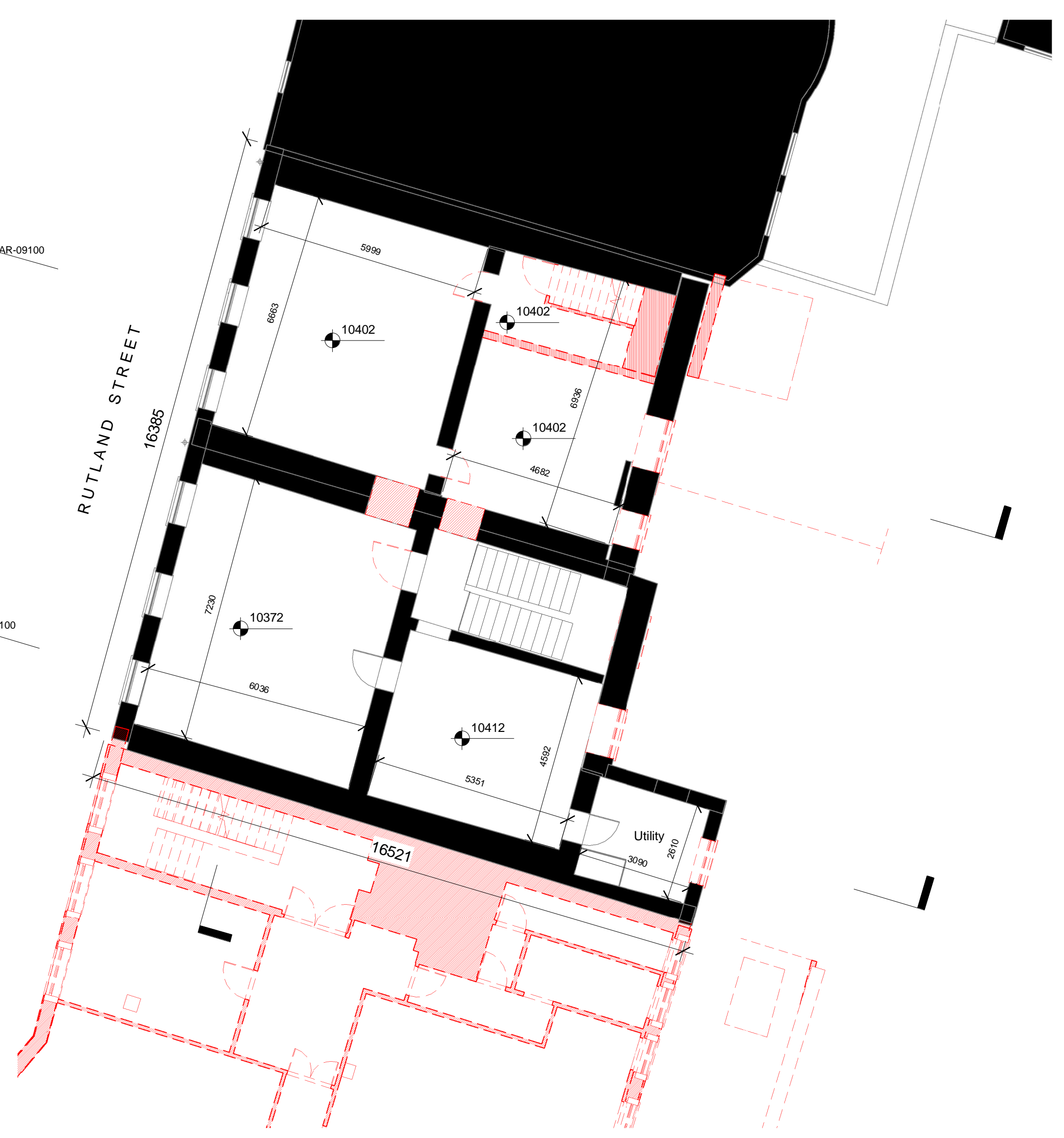
1 Demolition First Floor Plan SCALE: 1 : 100
